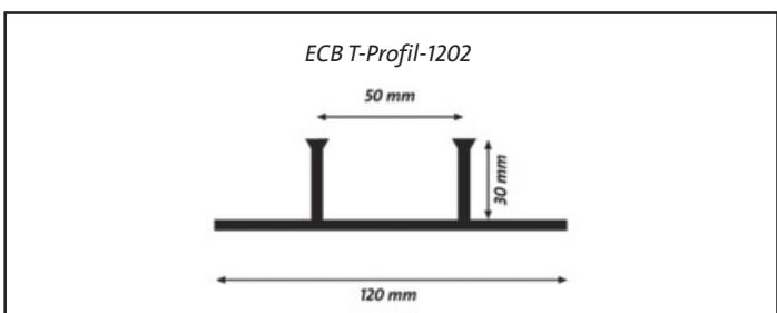
**EN** KÖSTER T-Profile types are manufactured from a special blend of highly flexible ECB using a high pressure extrusion process. The ripped side of the profile is cast together with the concrete and after the concrete cures it forms a very strong and waterproof bond with the concrete.
