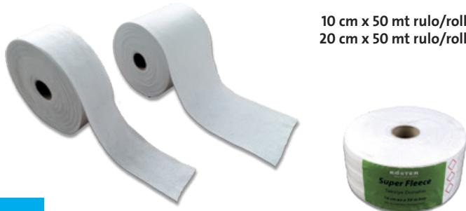
EN KÖSTER Super Fleece 120 is a non-woven fleece which is used as a reinforcement for liquid applied waterproofing materials. KÖSTER Super Fleece 120 quickly absorbs the liquid applied waterproofing material and cures together to form a highly tear resistant, crack bridging and waterproof fleece lamination.
