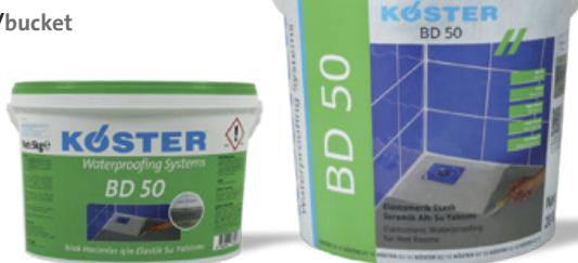
**EN** KÖSTER BD 50 is a one component, ready to use, solvent free, brushable coating for under tile applications in wet and damp rooms. The coating cures to a seamless membrane with high elasticity and crack bridging properties.
