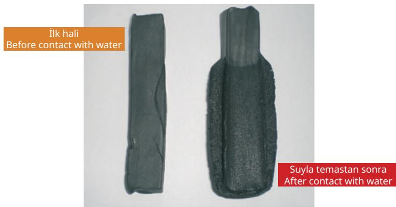
EN KÖSTER Quellband 2520 is a sodium bentonite based water swellable joint tape that swells upon contact with water to form a long lasting seal in concrete cold joints. KÖSTER Quellband has an alkalinity activated surface coating which stops premature swelling of the tape on the building site.
